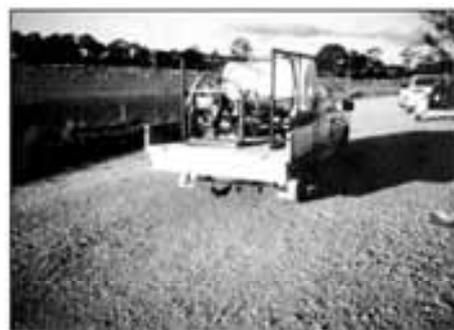
*Have a well-maintained firefighting unit at all times in the area where the burn-off is taking place.*
